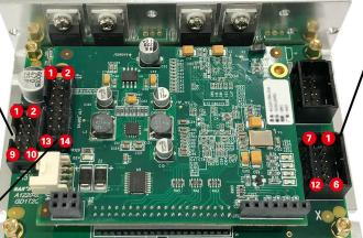
J2: Galvo signal control port Pin1: MOTOR1+ Pin2: -15V Pin3、4、5、9:GND Pin6:M1\_T+(Preheating circuit control end) Pin7: MOTOR1- (dangling) Pin8:HEATER1 (Preheating circuit detection end) Pin10:LED\_AGC (Photocell voltage detection terminal) Pin11:POS1\_IN-Pin12:POS1\_IN+
